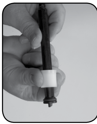
Step 4a for (TD100 - 1% & TD200 - 0.5%) Replace #44 DOSAGE PISTON flared-end up and #14 O-ring.
