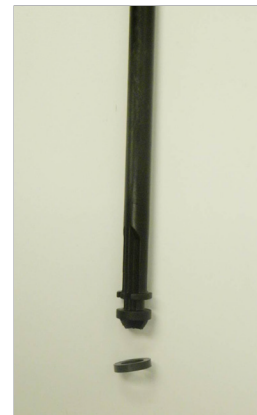
Step 3. Remove shaft with gasket and install new. If damage on sealing surface of shaft, replace shaft.
