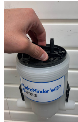
Step 6. Place new motor piston carefully into pump body and replace lid.
