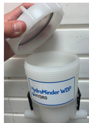
Step 9. Replace lid onto the pump body. Ensure o-ring is still in the lid before putting it back on.
