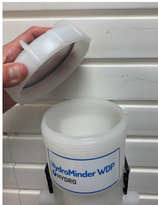
Step 4. Hold body firmly and unscrew the lid. If lid is tight, use 1" (25 mm) socket to loosen.
